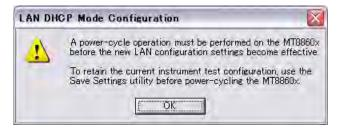
Figure 15-9. LAN DHCP Mode Configuration Warning
