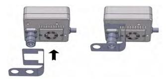
Figure 1. Rear of MN8861A with Stabilizing Bracket
