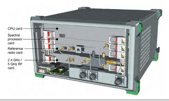
Figure 1-3. MT8860C Internal Structure
