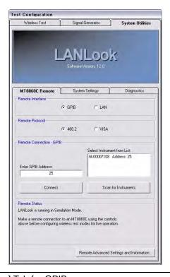
Figure 5-1. [System Utilities] Tab for GPIB
