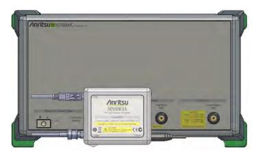
Figure 1-2. MT8860C with MN8861A Receiver Accessory
